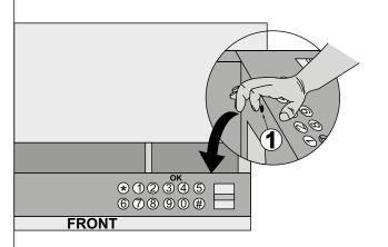
After opening the drawer safe using the fingerprint reader or factory security code, press the **RESET** button (1) until you hear a short "DI" signal. Then re-enter the factory unlock code 1234 and confirm using #. **OK** will be displayed. You can now enter your individual unlocking code (4 to 6 digits) and confirm with #. The code should be repeated and again confirm with #. If the code is accepted, **OK** will be displayed. Your new safe unlock code is now active.
