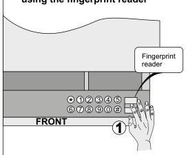
If the drawer safe has been previously programmed with an individual user code, it needs to be unlocked and opened with that same code, then the RESET button must be pressed until you hear a short 'DI' signal. Next insert your individual unlocking code again and confirm with #. Now place your finger (1) on the fingerprint pad, 'OK' will flash with a short "DI" signal, now repeat with your finger 3 more times. The display will go to standby. Your fingerprint is now active to unlock the safe.
